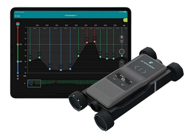
Profometer Rebar Diameter & Cover Meter
