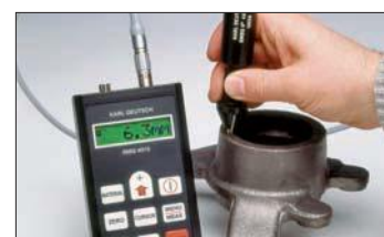
Measurement of a normal crack on a small area
