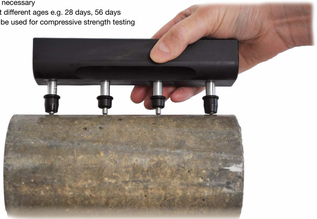
Resipod with 1.5" (38mm) probe spacing is fully compliant with the above mentioned standard
