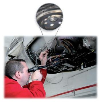
The 3.3mm allows inspection of narrow holes with tight bending curves.
