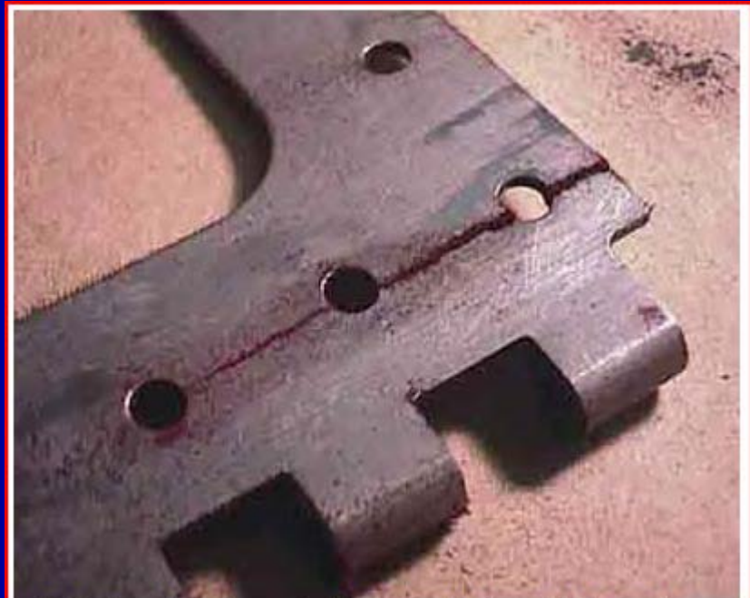
Indication of cracks running between attachment holes in a hinge
