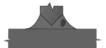
38 Slag Inclusion in Fillet (root area) UT, RT
