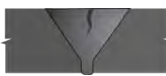
16 Circumferential Crack in Single Vee, flush crown MT/PT, UT
