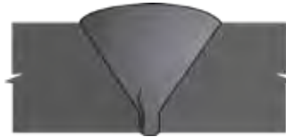
12 Root Crack in Single Vee MT/PT, UT, RT
