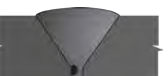
36 Slag Inclusion in Single Vee (root area) UT, RT
