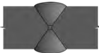
57 Incomplete Root Penetration in Double Vee, UT, RT
