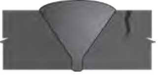
18 Base Metal Crack in Single Vee (top HAZ area) MT/PT, UT
