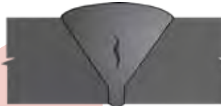
15 Centerline Crack, Single Vee (sub-surface) UT, RT
