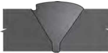
59 Incomplete Groove Weld (crown area) VT, MT/PT, UT, RT
