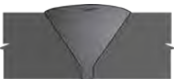
20 Crater Crack (crown stop-start area) MT/PT, UT
