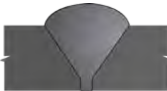
74 Excess Crown in Single Vee, VT
