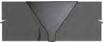
19 Base Metal Crack in Single Vee (bottom HAZ area) MT/PT, UT
