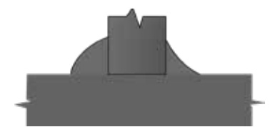
75 Excess Crown in Fillet, VT
