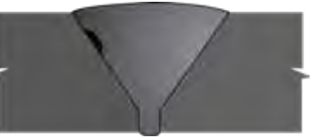
52 Lack of Fusion in Single Vee (crown area) UT
