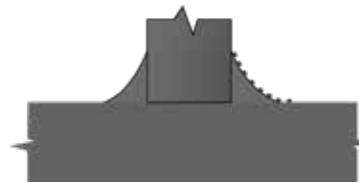
91 Weld Splatter on Filler VT, RT
