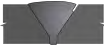
53 Lack of Fusion in Single Vee (surface breaking at crown) MT/PT, UT
