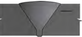
50 Lamination in Single Vee (base metal) UT
