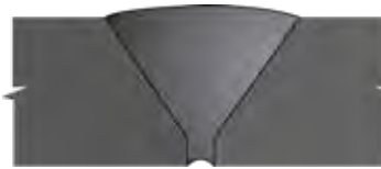
70 Root Concavity in Single Vee VT, RT
