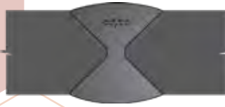
30 Porosity in Double Vee (sub-surface) UT, RT
