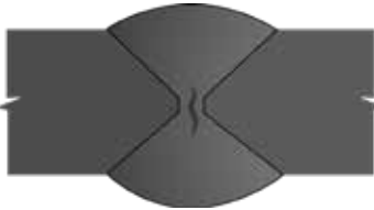
15 Centerline Crack in Single Vee (sub-surface) UT, RT
