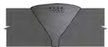
30 Porosity in Single Vee (sub-surface) UT, RT
