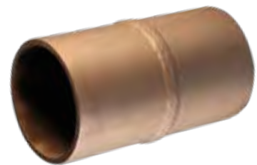
WELDED PIPING 4" SCH160(0.53"T)x 8" #P109
