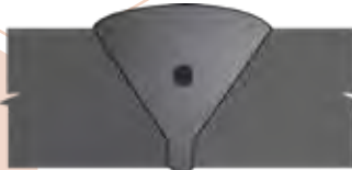
34 Single Gas Pore in Single Vee UT, RT
