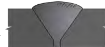
92 Chipping Hammer Marks on Single Vee, VT, RT
