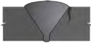
10 Toe Crack in Single Vee MT/PT, UT
