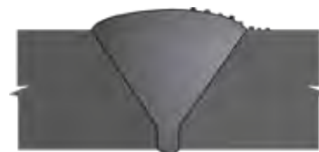
90 Weld Splatter on Single Vee, VT, RT
