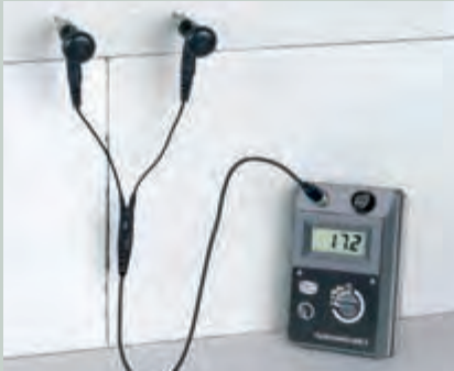
APPLICATION TIP Ideal electrode clearance: 10 cm
